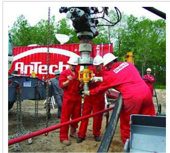
The team rigs up COLT BHA during the first well test. (Images courtesy of AnTech Ltd.)
